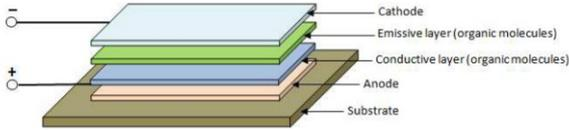
Fig. 1. OLED structure
