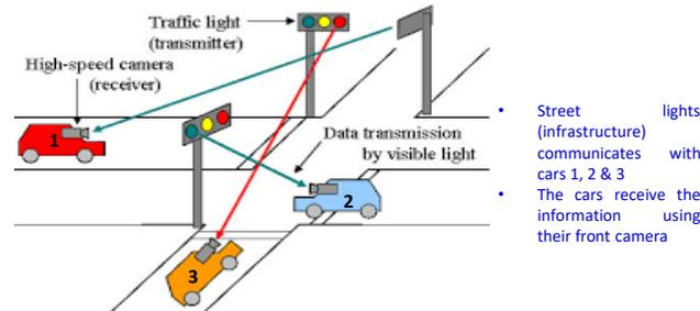
Figure 3: Infrastructure to vehicle communication [2]
