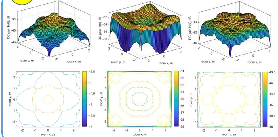
Figure 6: LOS DC gain of the transmitted optical beam at the receiver plane
