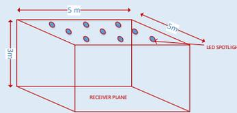
Figure 5: Modelled indoor VLC configuration
