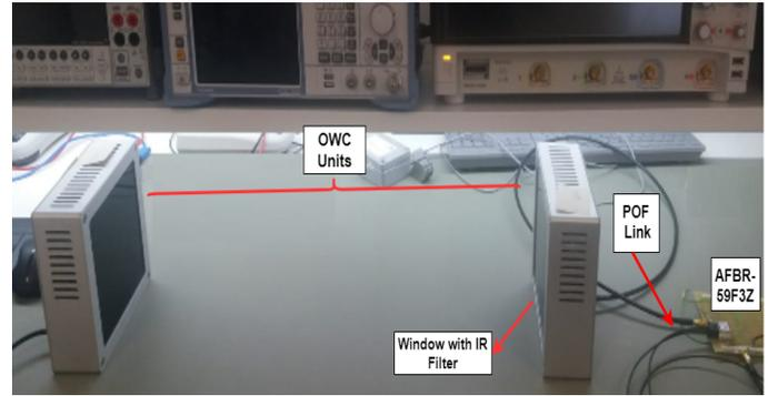
Fig. 4: Hardware implementation of POF and OWC link including AFBR-59F3Z and two OWC units with a point-to-point configuration is shown. The POF link has 2 meters length and both OWC units are configurable to act as an access point or as a client which, can operate for distances over 10m.
