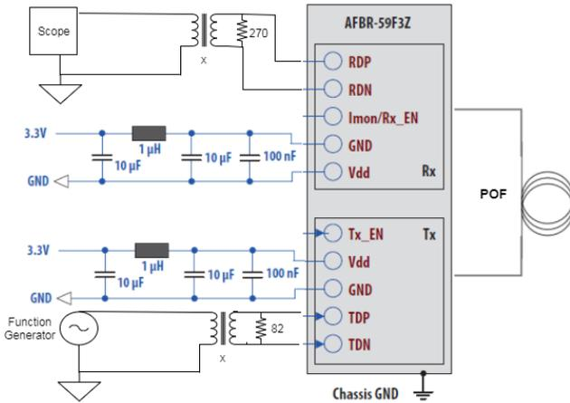
Fig. 3: Schematic of circuit measurement setup to establish the POF link. It shows the external circuitry for DC-coupling connection to power supply, function generator and oscilloscope.
