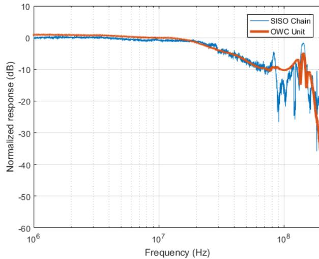
Fig. 8: Frequency response of the OWC unit alone and integrated with the POF link.
