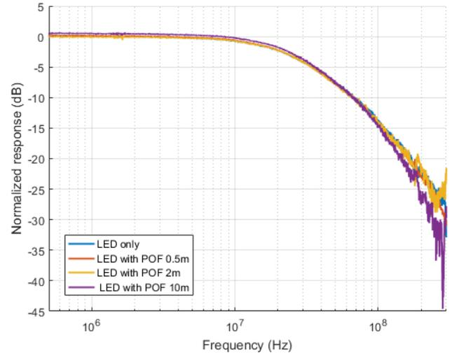
Fig. 6: Frequency response for the LED only and the LED including POF for various fiber lengths, all measured with a wideband reference photoreceiver in the lab. The response for 2 m POF connected to a first custom-designed POF receiver as shown in figure 3.
