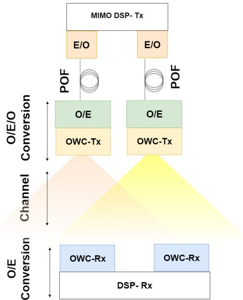
Fig. 2: In this paper, analog transmission of OWC signals over POF is investigated. The diagram shows the downlink only for simplicity, the uplink works similarly.
