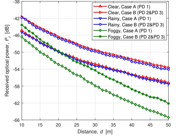
Fig. 4. Performance improvements due to dual photodetector deployment
