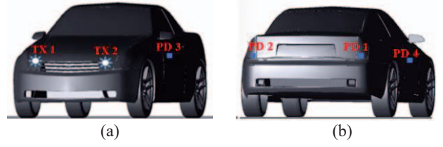
Fig. 2. Locations of high-beam headlights (transmitters) and photodetectors (receivers) on the vehicles.
