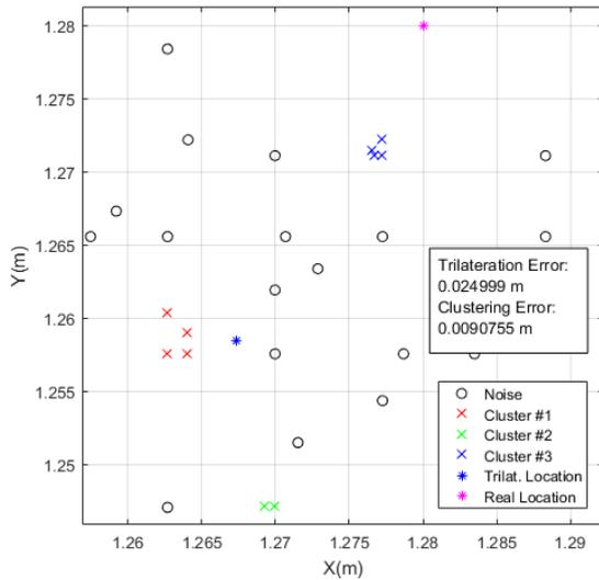
Fig.4 Formation of cluster using machine learning algorithm (reprint with permission from [29]).
