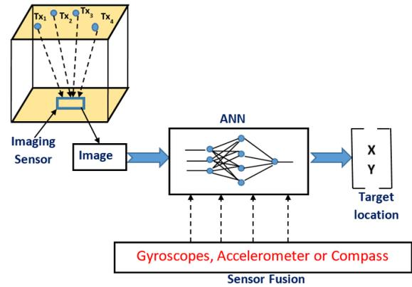
Fig 5. Setup for ANN and sensor fusion.
