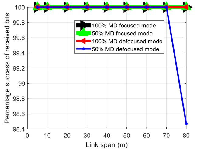
Fig. 7. Success rate of the data transmission over a link span for the focused and defocused camera modes
