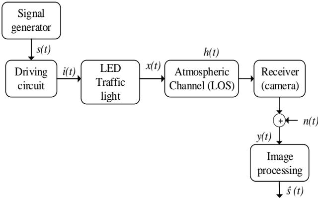
Fig. 1. The schematic block diagram of a VLC-based V2I system.
