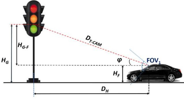
Fig. 2. Configuration of the V2I VLC system
