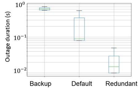
Fig. 8: Outage duration for mobility usecase scenario in a VVLC network.
