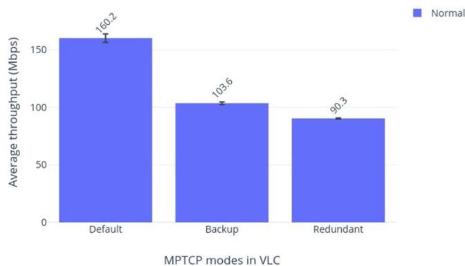
Fig. 3: Average throughput of MPTCP in VLC links using "Default", "Redundant" and backup-mode MPTCP tool.
