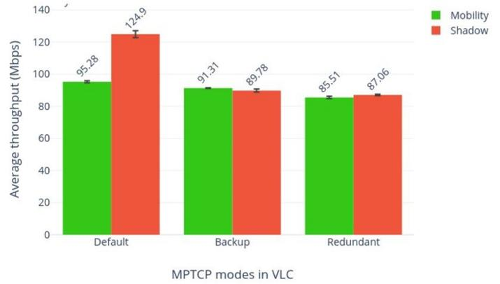
Fig. 7: Overall average throughput of MPTCP on mobility and shadow usecases.
