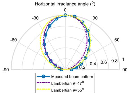
Fig. 2. Measured and Lambertian radiation pattern.
