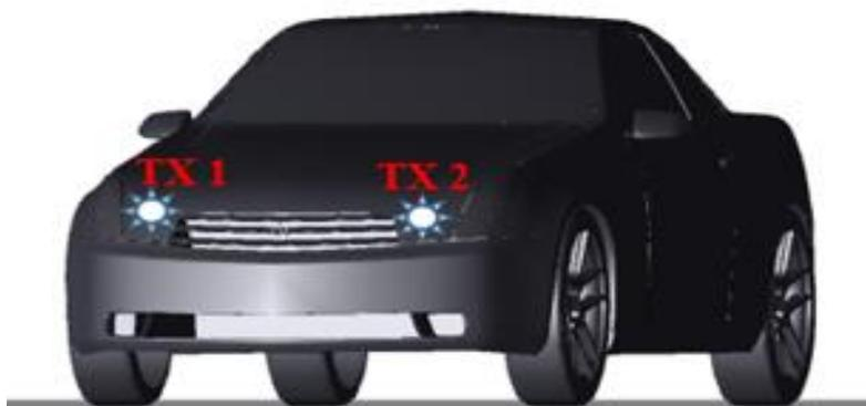
**Fig. 5** Location of transmitters on the car
