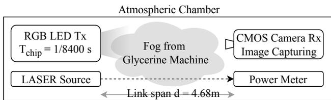
Fig. 2. Diagram of the experimental setup.
