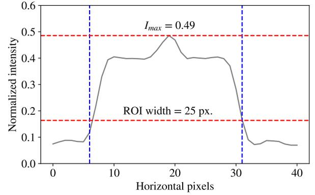
Fig. 3. Output from the estimation of ROI dimensions of an example test signal. Red lines are: (upper) peak intensity, and (lower) the decay of 20% of the extinction ratio. Blue lines are the intersection of red lines and the grayscale intensity profile of lamp (horizontal axis).
